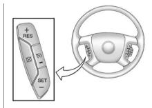
The cruise control buttons are located on left side of the steering wheel.
